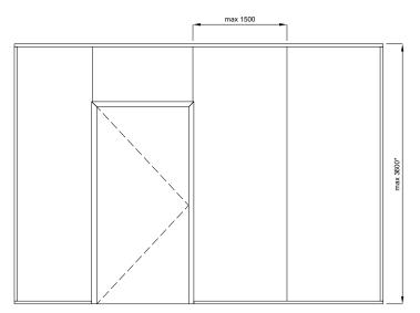
\* - for glass types VSG 66.1, VSG 66.2, VSG 66.2 and VSG 66.2 with acoustic film, ESG 12 mm
