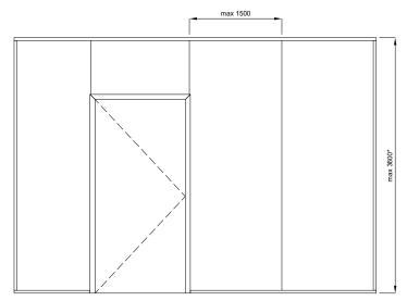
$<sup>^{\</sup>ast}\,$  - for glass types ESG 12, VSG 66.1, VSG 66.2 and VSG 66.2 with acoustic film
