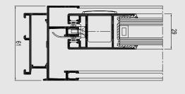
The CP 45Pa is a non-insulated sliding system that has been designed to respond to new aesthetical demands. The system is available in functional and softline design. The profile width is reduced to a minimum allowing a maximum of light into the building.
